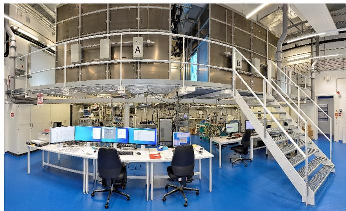
**Figure 4.** Atmospheric Chemistry Department – Chamber (ACD-C) allowing the investigation of toxicological effect of aerosols
