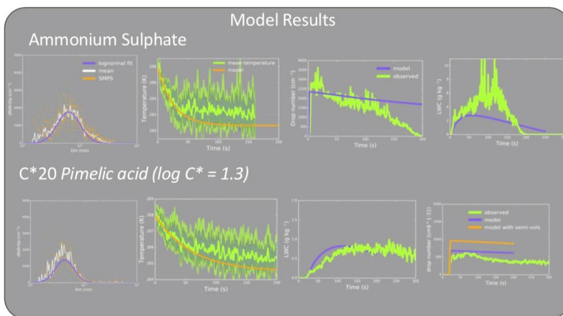
**Figure 10:** PyACPIM GUI snapshot showing warm cloud activation on ammonium sulphate and semi-volatile organic particles, comparing simulated with experimental data.
