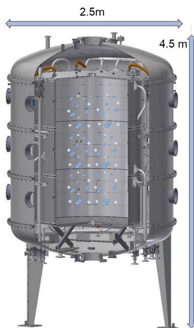
**Figure 3.** The new dynamic cloud simulation chamber AIDA for studying aerosol-cloud interactions
