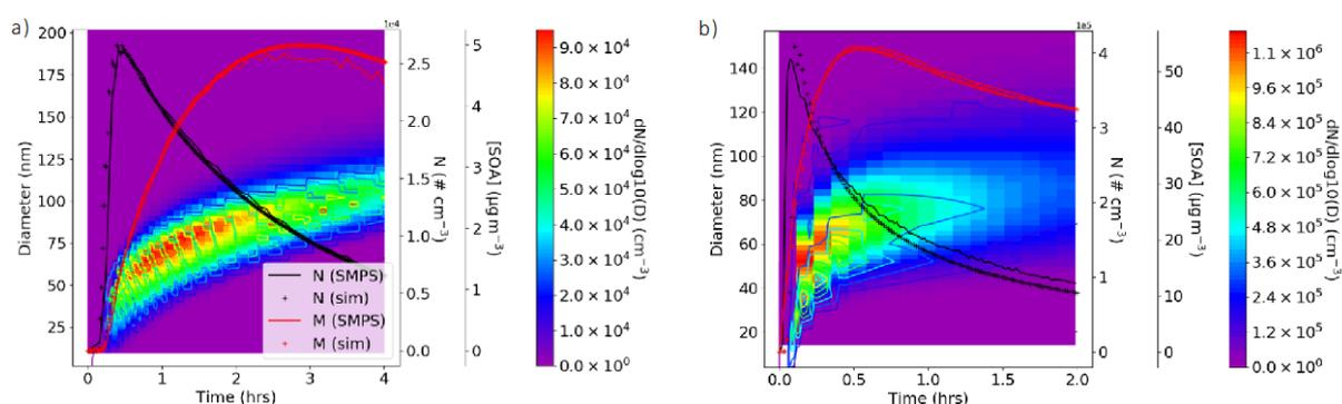
**Figure 9:** Simulated  $\alpha$ -pinene ozonolysis in MAC and AIDA using an extension appended to the MCM in PyCHAM, with only wall loss (with effective absorptive wall mass for vapours) tuned for each chamber. Measured and modelled number size distributions shown by filled and line contours respectively.
