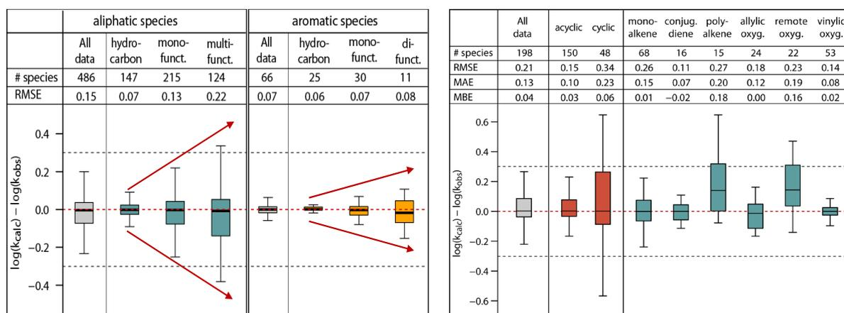
**Figure 7:** Root mean square error, mean absolute error, mean bias error and box plots for the error distribution in the estimation of  $k_{298K}$  values for OH (left) and ozone (right) reactions for a full set and subsets of the aliphatic (Jenkin et al., (2018a)), aromatic (Jenkin et al., (2018b)) and alkene (Jenkin et al., (2020)) species in the respective databases.
