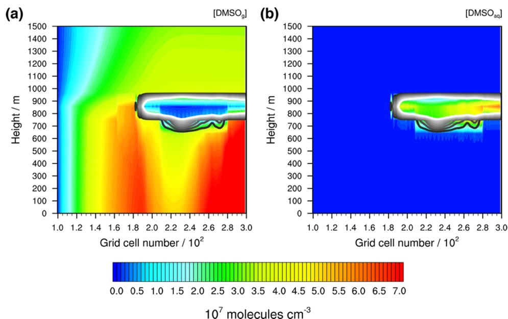
**Figure 8:** Simulated concentrations of DMSO (a) in the gas phase and (b) in the aqueous phase under stratiform cloud condition after 12 h of modelling time. The x axis represents the innermost horizontal grid cells divided by 100. The black contour lines represent the simulated clouds. The black line indicates a LWC of 0.01 g m<sup>-3</sup> and the white line to 0.1 g m<sup>-3</sup>. The area framed by the white line includes LWC above 0.1 g m<sup>-3</sup>.
