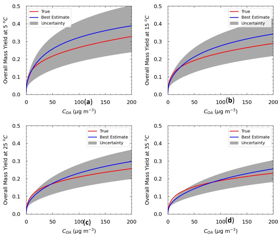
**Figure 11:** Yields calculated by the true (red) and estimated (blue) stoichiometric coefficients of a typical test of the algorithm at: (a) 5 °C, (b) 15 °C, 25 °C, and (d) 35 °C. The grey area represents the uncertainty range of the best fits.
