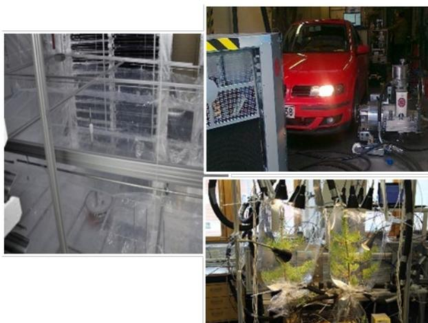
**Figure 5.** Chambers deployed to investigate vehicle emissions, eventually mixed with biogenic compounds
