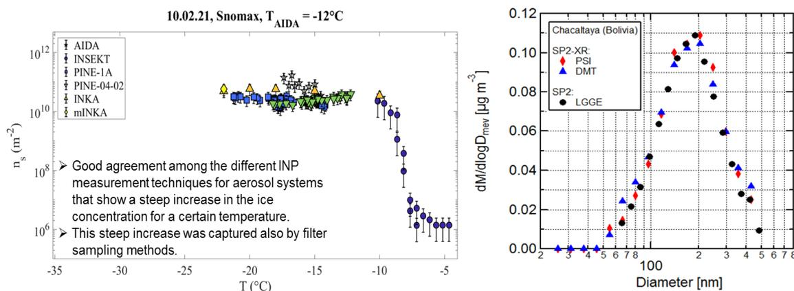
**Figure 1.** (Left) Example of methods developed at ACcloud for calibrating ice nucleating particles (INP) measurements. (Right) Example of excellent agreement of independent refractory black carbon (rBC) measurements achieved in a field study following calibration at CCSM.
