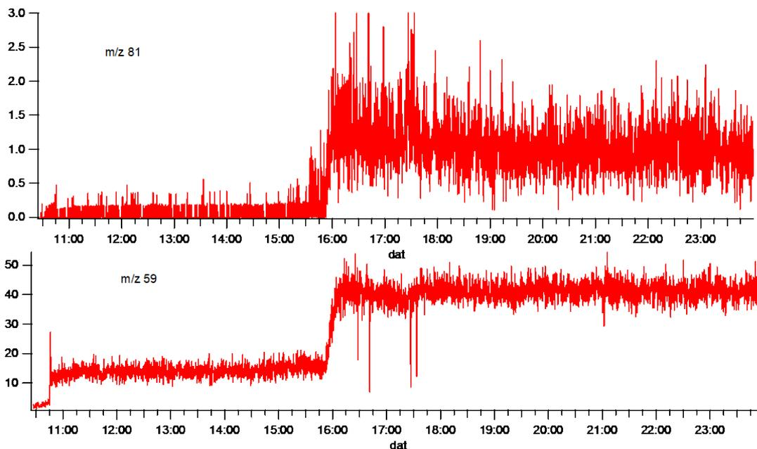
**Figure 3.** PTR-MS measurements of organic vapors during a typical Norpinic acid production. HONO was introduced in the chamber and the lights were turned on at 15:45.
