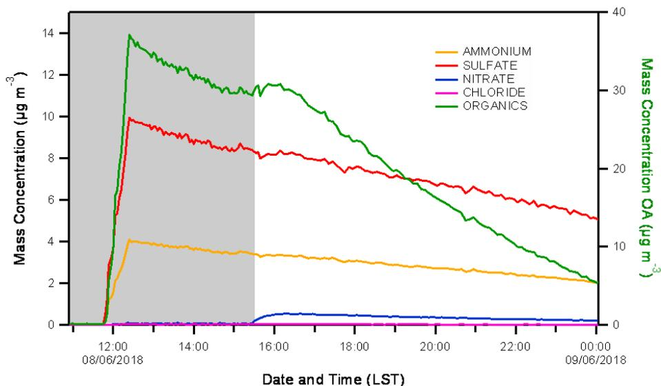
**Figure 4.** Aerosol composition for typical DTA experiment. The shaded area corresponds to the characterization phase of the fresh aerosol (lights-off), while the white area to the chemical aging phase (lights-on). HONO was introduced into the chamber at the beginning of the aging phase.
