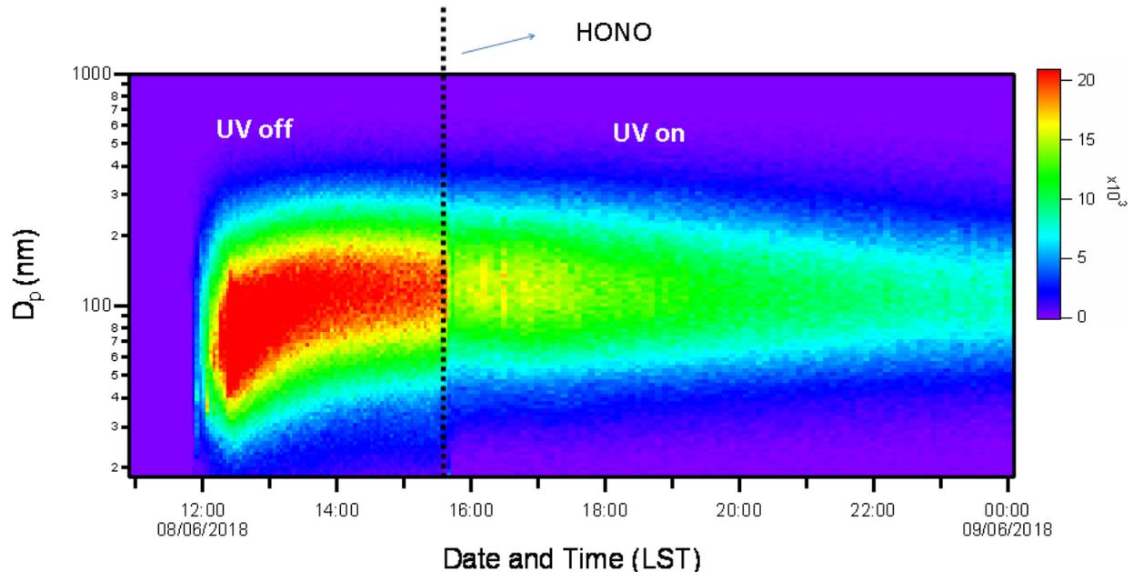
**Figure 5.** Typical aerosol size distribution during a DTA experiment. The two phases (initial characterization and aging) are shown.
