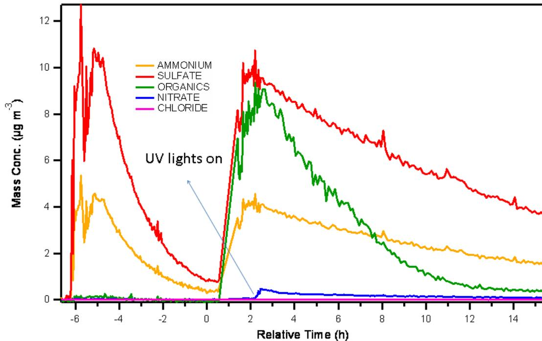
**Figure 7.** Aerosol composition for typical terebic acid experiment. The shaded area corresponds to the characterization phase of the fresh aerosol (lights-off), while the white area to the chemical aging phase (lights-on). HONO was introduced into the chamber at the beginning of the aging phase.
