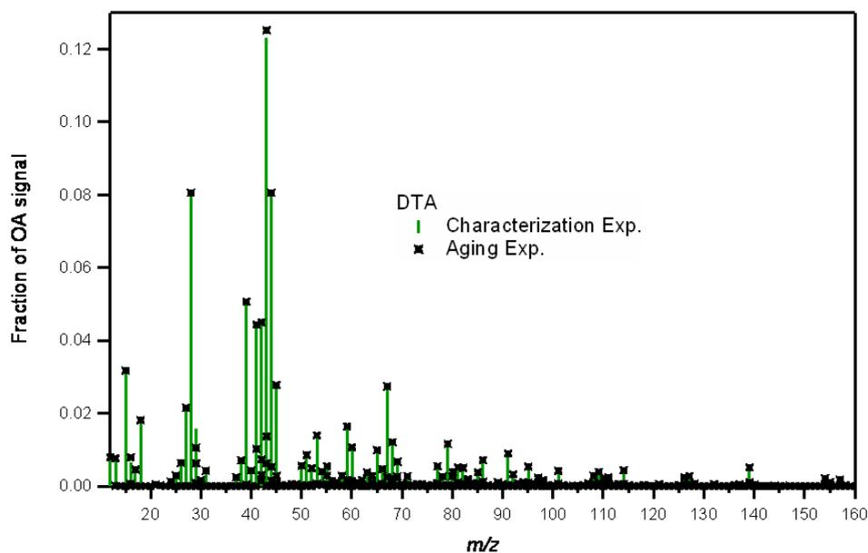
**Figure 6.** AMS spectrum of fresh DTA and of DTA after exposure to OH for several hours. The changes were minor.
