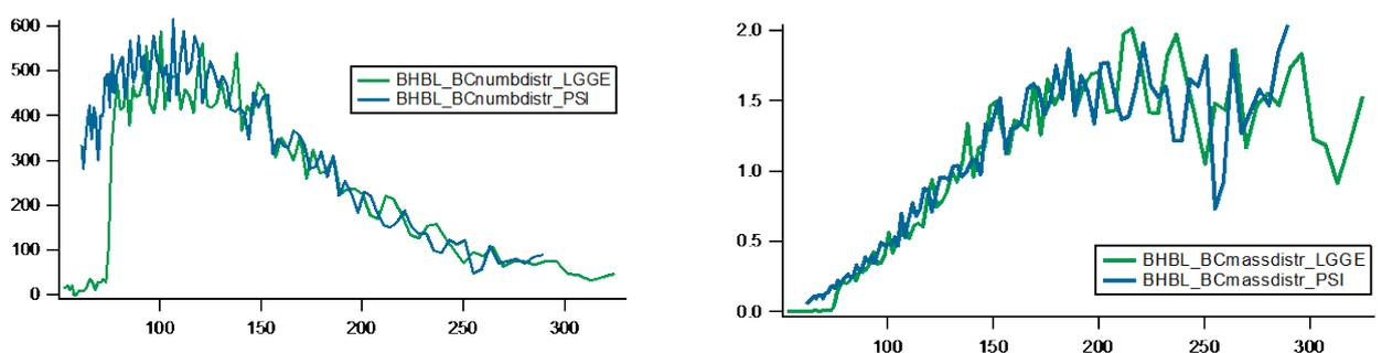
The scattering size distribution is consistent only in diameter range from 250 to 400 nm, that could be due because of the different detector used (HG in LGGE vs Split in PSI).
