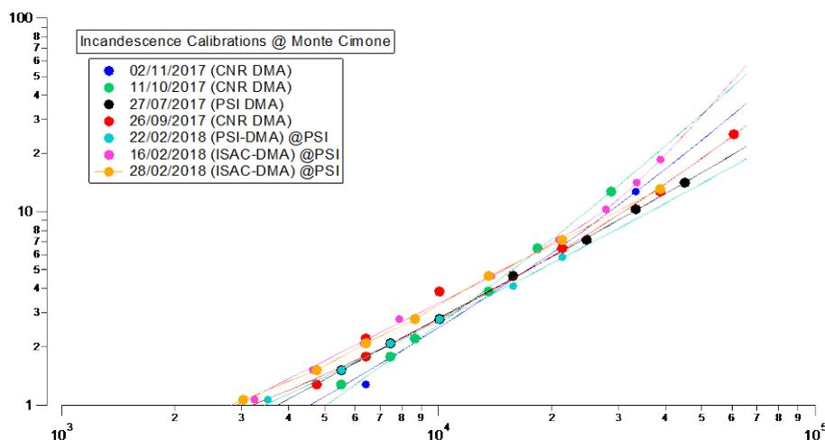
Figure 1. Comparison of broadband incandescence channel during incandescence calibrations performed at Monte Cimone and PSI.
