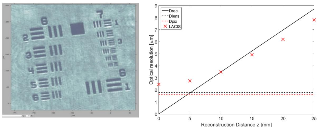
( $D_{rec}$ ) is plotted in Fig. 2. The fig. also shows that experimental and theoretical values are in a good agreement. It can be concluded that the determined lower detection limit of  $2.46 \mu\text{m}$  at the focal plane is a great improvement by a factor of about 8 compared to the detection limit of the holographic system without any magnifying lens. It is also an improvement compared to the  $7 \mu\text{m}$ , which can be achieved at the MTU Pi chamber (at a longer working distance).
