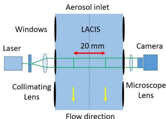
required to confidently distinguish a particle/droplet from the background image, the lower detection limit without any further magnification is (at least) 20  $\mu\text{m}$ . The detection limit was improved by installing a magnifying optics with a magnification of 12.5. The optics consists of a telephoto lens and a 2x magnification lens (NTX Tube 2x).
