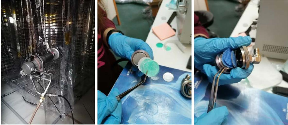
*Testing filtration efficiency of materials for mask production to help protect the medical and broader community in FORTH, Patras.*
