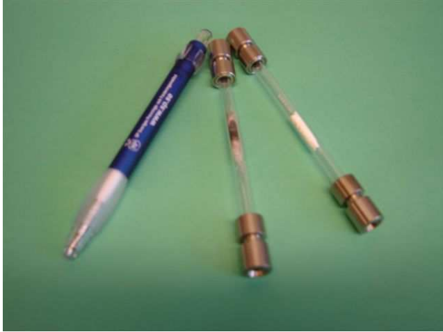
Picture of the thermodesorption tubes with a powder sample (left) and a filter sample (right)
