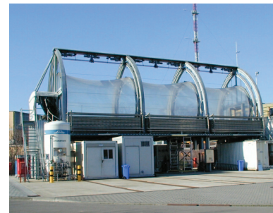
The SAPHIR simulation chamber at Jülich Research Centre, Germany
